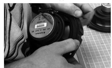
NOTE: You can insert the one side of the speaker into the assembly and use a flat bladed screwdriver or pry bar to gently pry the grille onto the speaker for a tight fit. Be sure to orientate the speaker with the terminals up.
