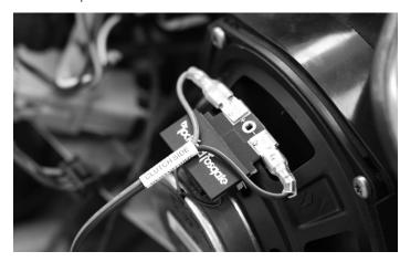
NOTE: The terminals utilize the 1/8" for negative (-) and the 1/4" for positive (+) sizing for easy connections.
