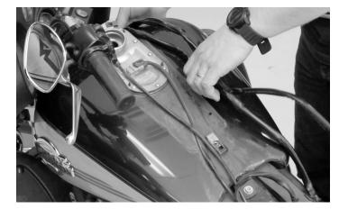
\*\* WARNING The gas cap should not be left off. Once the console is off put the cap back on to prevent any gas fumes creating a potential fire hazard.
