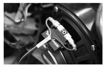
NOTE: The terminals utilize the 1/8" for negative (-) and the 1/4" for positive (+) sizing for easy connections.
