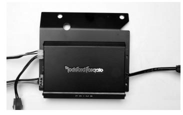
Mount the bracket to the brake side turn signal bracket. Once the amplifier is mounted, you can now wire up the speakers.
